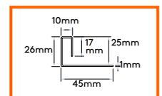
Use vertically at the end of a cladding run to butt the boards against, protecting the weatherboard & giving a straight edge framing to the clad area. The End profile 65 will also cover the 38mm batten if your cladding leaves this exposed.
