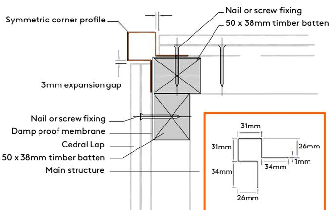
Use on vertical corners where lapped boards are being installed on either side of the corner.
