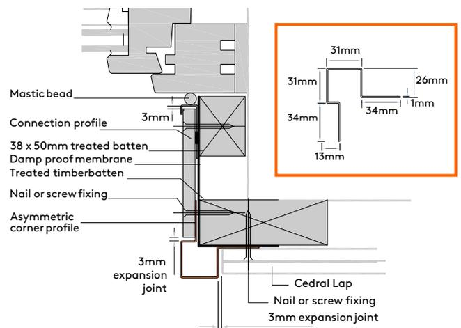
Use on right and left vertical of windows and doors allowing for lapped boards on face side of building and single board laid flat around the reveal of window or door.
