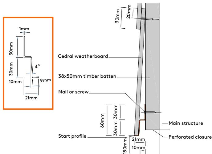
Use to kick the board out along the first bottom run of cladding and also above any windows or doors.
