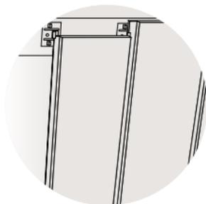
EDPM must be used on the front face of all horizontal trapezoidal battens.
