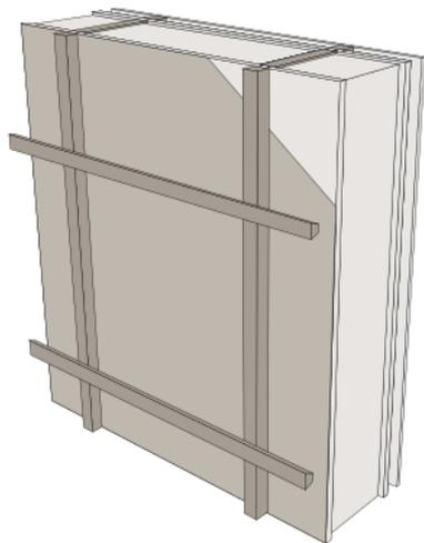
Horizontal counter battens should then be fixed.
