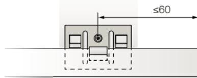
The distance from the edge of the Click Clip to the edge of the Cedral plank should not exceed 60mm
