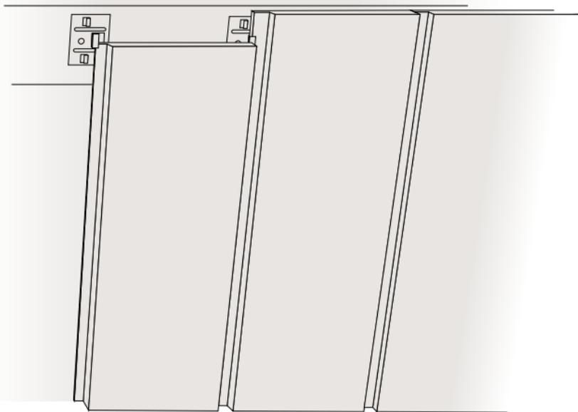
Screw Click Clips onto every batten to fix the edge of the plank into place.
