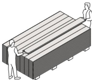
Planks must be lifted off the stack
