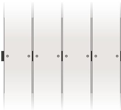
Planks are laid next to each other, with a 3-12mm open gap between each.
