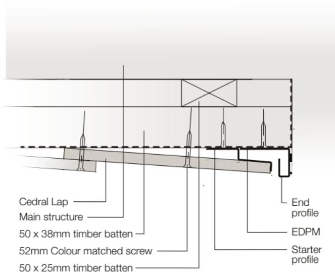
Place secondary fixings through the tail of the plank at 50mm from the edge and fixings are every 600mm (these will remain visible).
