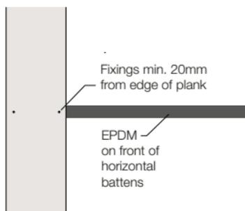
Loosely butt joint the next plank or leave a uniform gap of between 0 and 2mm between planks. Screw into place in the same way.
