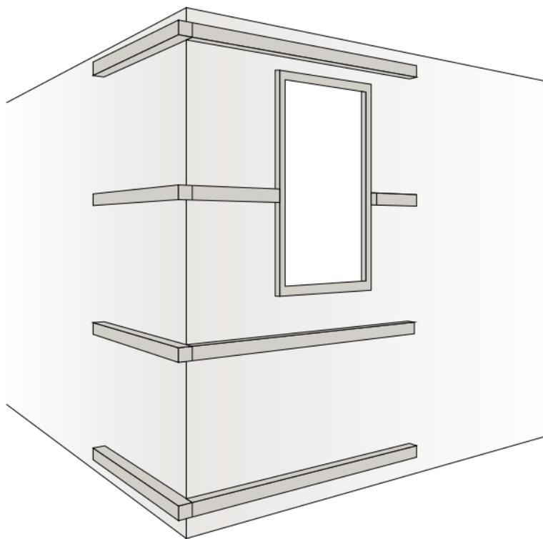
\* For solid walls, timber frame and metal stud constructions it is good practice to include a breathable membrane behind the battens. Generally for unfilled/partially filled cavity walls there is no requirement to do this.
