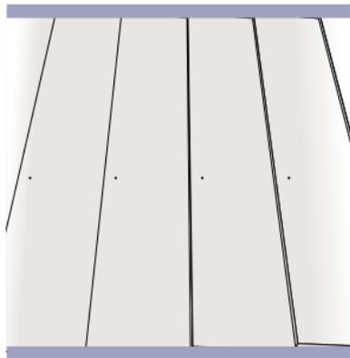
Install horizontal end profiles at the top and bottom of each section of cedral planks. Drill weep holes to allow for drainage.
