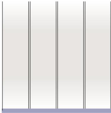
Fix vertical start profile below all Cedral Click planks to support the system. Vertical start profiles are required at every 3.6m for every row of new planks.
