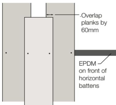
Screw through the face of the front planks penetrating both planks and screwing into the timber. Fixings must be 20mm minimum from the edge of the plank and again all planks must be fixed twice to every batten.
