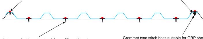
Main fasteners that incorporate minimum 29mm diameter sealing washers @ maximum 200mm centres. Minimum 19mm diameter washers may be used with a CE36E, CEDR30E or Supasafe E sheet, subject to wind loads
