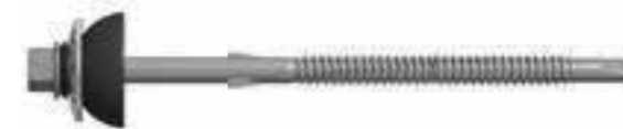
105mm screws for thin Zed purlins between 1.6mm and 2.5mm - DF3 -FCW 5.5 x 45 (75 for vertical).
