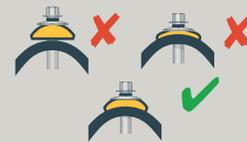
To achieve a watertight and weathertight seal, it is important to confirm that the sealing washer is correctly tightened. **Not over tight, not too loose.** After a period of time, when the material has settled, the fixings may require re-tightening with hand tools. Be sure to use roof ladders to avoid walking on the roof sheets.
