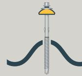
It is extremely important that the correct roof purlins/rail system, type of fixing and washers are selected, to eliminate leakage/corrosion and the general deterioration of the construction. It is recommended that a self-drilling Top-Fix screw is adopted. This simple method offers a fast, low-cost fixing solution. Using a high-speed screw gun, drive in the fixing. The fixing system is only suitable for roofs up to and including 30° pitch.
