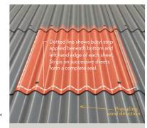
Butyl strip is shown in dotted white beneath the Cemsix sheet (coloured orange for clarity) and in solid white below the (grey) Cemsix sheet in the next course above and below the adjacent (grey) sheet to the right.
