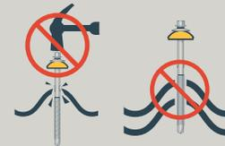
NEVER hammer fixing through the sheet. This will invalidate the guarantee. Fibre-cement sheets will shatter under impact and subsequently allow water to penetrate the apparent fixing. ALWAYS pre-drill.
