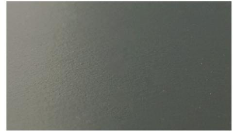
**POLYESTER PAINTED** is a factory applied 2-part paint coating applied to a fully galvanised substrate offering a fully functional yet highly cost effective finish.
